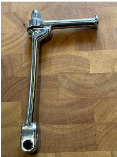
Burman Folding Kickstart, 194-X-39 (G-43-8) Listed for one year, one model only – 1951 C. Very good condition and splines. NB offset is only \frac{3}{4} "
